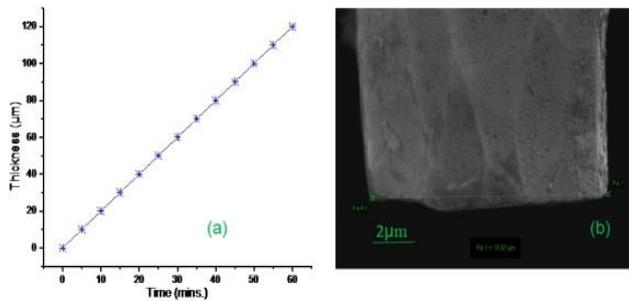
Figure 5. (a) Variation of the tip diameter with etching time and (b) Cross-sectional SEM image of the probe tip (diameter: 7  $\mu\text{m}$ ; average etching time: 15 min), which demonstrates complete Polyvinylidene fluoride (PVDF) encapsulation through the electrospinning on fibre surface (scale bar, 2  $\mu\text{m}$ ).
