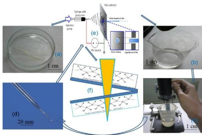
Figure 1. Schematic illustrations of HMCE technique (a) Raw fiber after cleaning (scale bar, 1 cm), (b) Fiber dipped into acetone to remove the jacket (scale bar, 1 cm), (c) Selective chemical etching technique (scale bar, 1 cm) (Microscope was stepping in upward direction) (d) Pencil shaped tip (scale bar, 20 mm), (e) Electrospinning process and (f) Polyvinylidene fluoride (PVDF) encapsulation.
