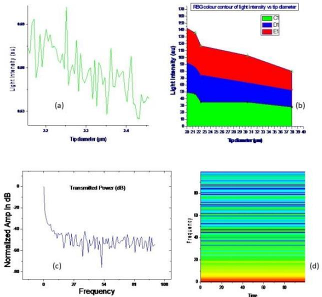
Figure 6. Light intensity as a function of tip diameter of the fabricated probe at 632.8 nm incident wavelength of (a) Transmission spectrum of LASER beam through the tip of the fiber, (b) RGB color contour of transmitted optical output in terms of fundamental color spectra, (c) Normalized transmitted power amplitude in dB and (d) STFT of the signal.
