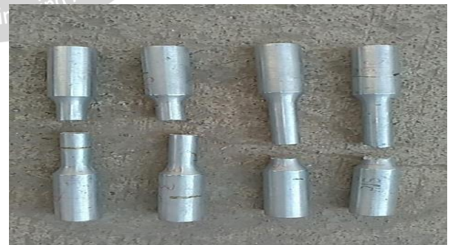
Fig: 12 Fractured AA 7178 specimens
