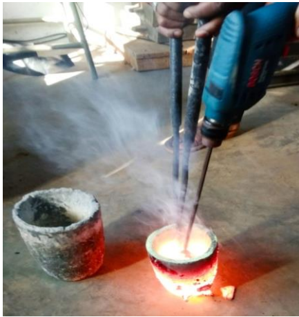
Fig.2 Shows Schematic diagram of Stir Casting technique
