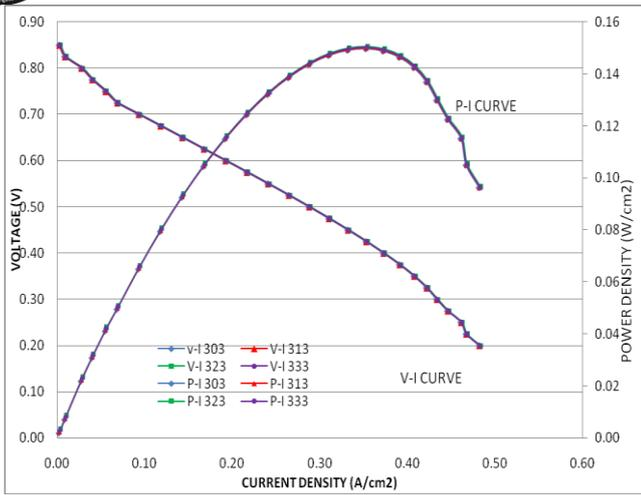
**Fig. 2. Polarization and Performance curve of 81 cm<sup>2</sup> serpentine flow channel with various temperatures with 1 bar pressure**
