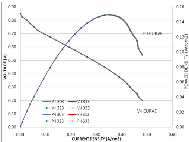
**Fig. 3. Polarization and Performance curve of 81 cm<sup>2</sup> serpentine flow channel with various temperatures with 2 bar pressure**
