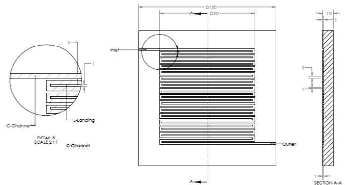
**Fig. 1. 2D model of serpentine single pass flow channel of 81 cm<sup>2</sup> active area with Landing to Channel ratio of (L:C) – 2:1**
