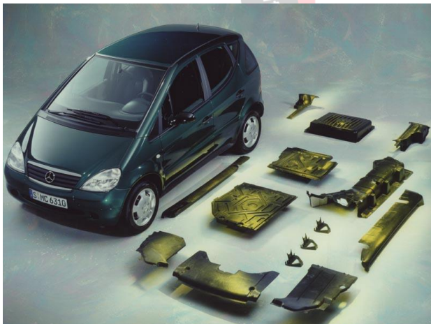
Figure3: Mercedes Benz use of Abaca fibres in parts
