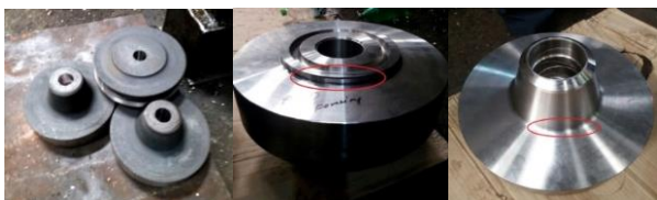
Figure 1: Unfilling defect at job
