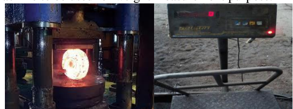
Figure 2 & 3: Hammering Operation & Electronic Weighing Machine respectively
