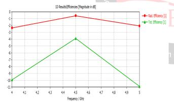
The radiation efficiency is found to be approximate -1.52dB at 4.5GHz and -2.062dB at 5GHz. The total efficiency is found to be -4.02dB at 4.5GHz and -10.87dB at 5GHz.
