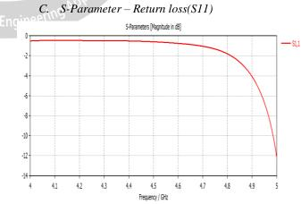
In this analysis, the return loss is monitored between 4GHz and 5GHz. It is found that the return loss value remains consistent at approximately -0.8dB up to 4.5GHz and the major dip occurs a little beyond 5GHz with nearly -14dB.
