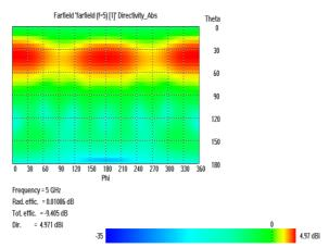
The far-field directive radiation at a frequency of 5GHz is 4.97dB.
