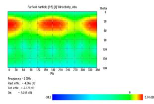
The far-field directive radiation at a frequency of 5GHz is 5.74dB.
