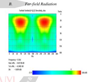
The far-field directive radiation at a frequency of 5GHz is 8.06dB.
