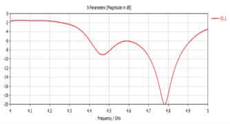
The sudden dip occurs at 4.78GHz with -20Db and nearly reaches -4dB at 5GHz.
