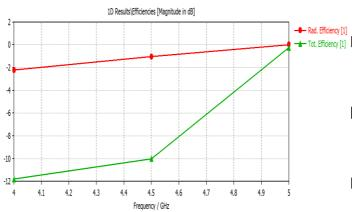
The radiation efficiency is found to be approximate -1.25dB at 4.5GHz and 0.02138dB at 5GHz. The total efficiency is found to be -10.02dB at 4.5GHz and -0.2482dB at 5GHz.
