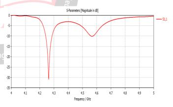
The sudden dip occurs at 4.27GHz with -30db and almost nears 0dB at 5GHz.
