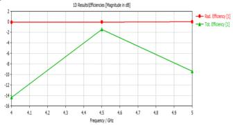
The radiation efficiency is found to be almost 0dB at 4.5GHz and 0.01086dB at 5GHz. The total efficiency is found to be -1.98dB at 4.5GHz and -9.405dB at 5GHz.
