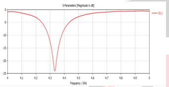
The sudden dip occurs at 4.34GHz with -24dB and around 1dB at 5GHz.
