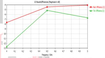
The radiation efficiency is found to be -4.4dB at 4.5GHz and -4.066dB at 5GHz. The total efficiency is found to be approximate -5.21dB at 4.5GHz and -6.679dB at 5GHz.
