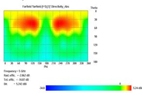
The far-field directive radiation at a frequency of 5GHz is 5.24dB.
