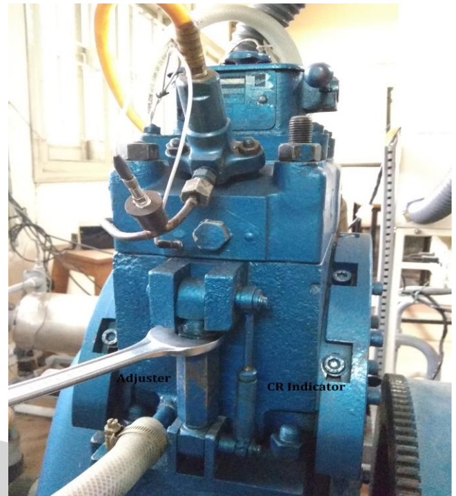
Figure 3: Variation of Compression Ratio using lock nut
