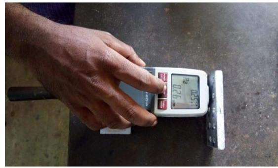
Fig.6 Measurement of Surface roughness
