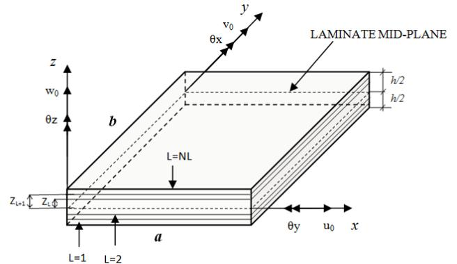
Fig. 1.0. Geometry composite laminated plate with positive set of reference axes and displacement components
