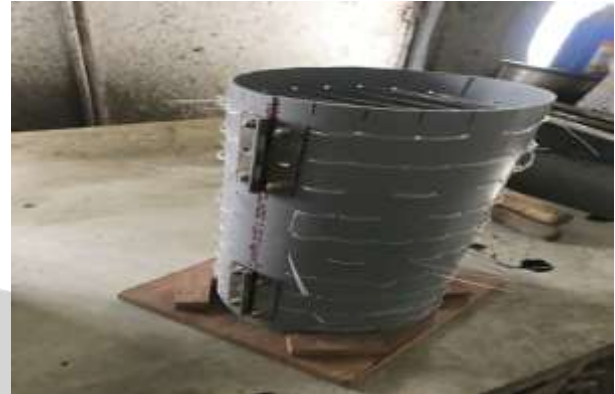
Fig.4.3 Cylinder (PVC) with plastic optical fibre
