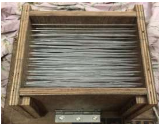
Fig.4.2 Wooden prism with plastic optical fibre
