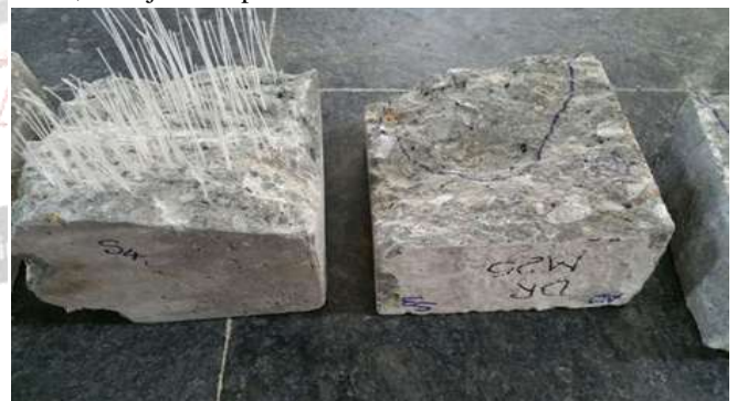
Fig.5.4 Water permeability test specimens
