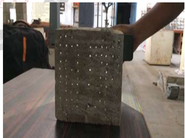
Fig.4.4 Transparent concrete after been cast
