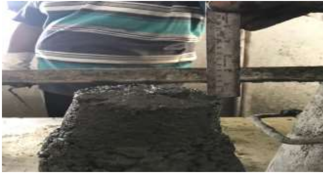
Fig.5.1 Slump cone test
