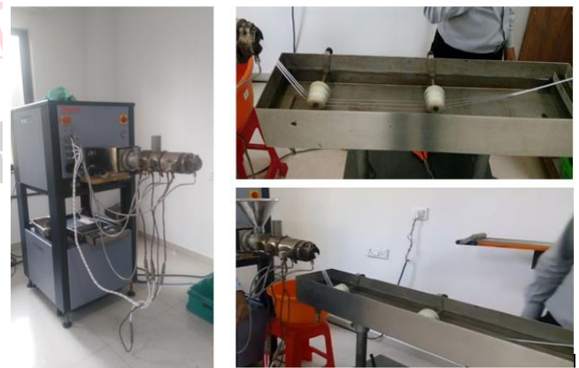
Figure 1: Preparation of LLDPE/COC blend using Haake Rheomix TW100.
