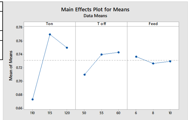
Fig 5.4 Effects of process parameter on means graph for kerfs width.
