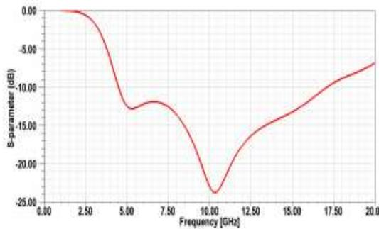
**Fig.24.Simulated absorption behaviour of proposed Broadband absorber using two Minkowski loops**
