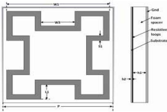
Fig.17. Unit cell of the absorber using single Minkowski loop
