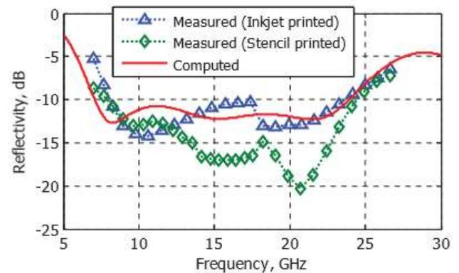
Fig.8. Simulated and measured reflectivity plots at normal incidence
