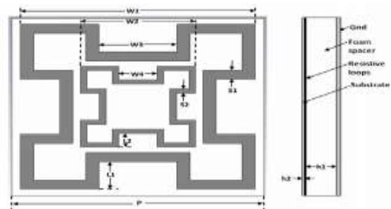
Fig.23. Unit cell of the absorber using two Minkowski loops
