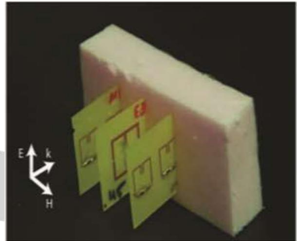
**Fig.3. Unit cell consisting of Lumped Elements**
