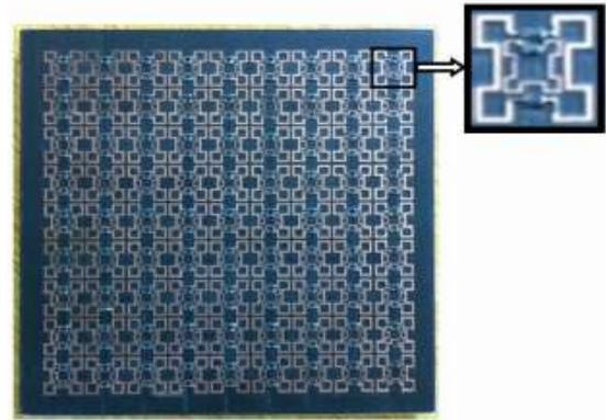
Fig.21. Prototype Broadband Absorber
