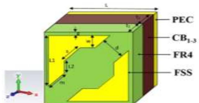
**Fig.1. Schematic representation of hybrid absorber with its various dimensions as,  $L = 10$ ,  $L_1 = 6.878$ ,  $L_2 = 1.878$ ,  $s = 2.828$ ,  $m = 2.121$ ,  $d = 3$ ,  $g = 0.5$ ,  $\omega = 1.5$ ,  $t_1 = 1.8$ , and  $t_2 = 0.8$  (all dimensions are in millimeter).**
