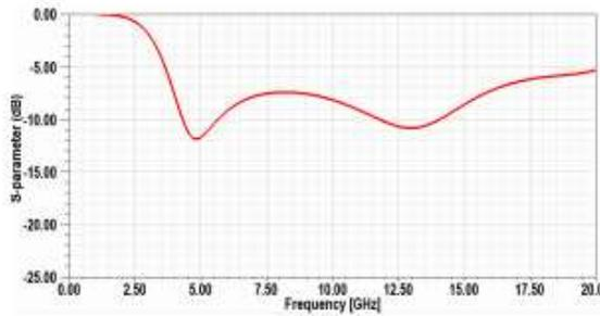
Fig.18. Simulated absorption behaviour of proposed broadband Absorber using single Minkowski loop
