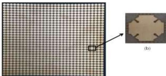
introduced in the four circular cross sector. Owing to the symmetric unit cells high absorptivity is maintained for all the polarization angles. Under oblique incidence the zero reflections for the TE and the TM modes are different and so the unit cell insensitive to the TE and TM polarization must be designed.
