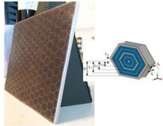
Fig.7. Photograph of the manufactured metal backed FSS absorber and schematic and dimensions of the FSS unit cell;  $p=6.9$  mm,  $L1=5.6$  mm,  $L2=4.2$  mm,  $L3=2.5$  mm,  $L4=1.1$  mm,  $w1=1.1$  mm,  $w2=1.2$  mm,  $w3=1.1$  mm,  $w4=1.2$  mm,  $R=27 \Omega/\text{sq}$ ,  $t_a=3$  mm,  $t_t=0.13$  mm
