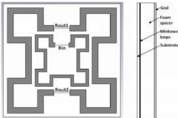
Fig.19. Unit cell of the absorber with only 3 resistors
