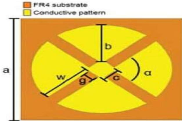
**Fig.13. Angle insensitive MM Absorber using four circular sectors**
