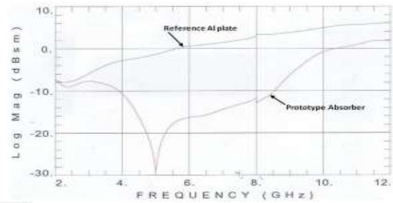
Fig.22. Measured RCS of prototype broadband absorber
