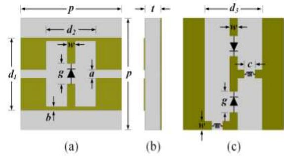
**Fig.9. Unit cell geometry of the proposed MAFSS (a) Top view of top layer, (b) side view, and (c) top view of bottom layer.**
