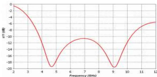
Fig.20. Simulated Reflection loss of the absorber with only 3 resistors per unit cell
