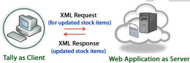
Fig 4.2: representation of data extraction from web application.
