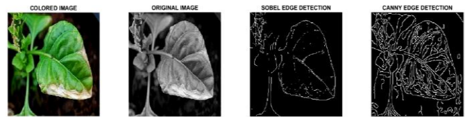
Fig: - Image pre-processing (Edge Detection Method)
