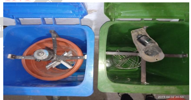
Fig.3: Top View of Compost Bin and Digester
