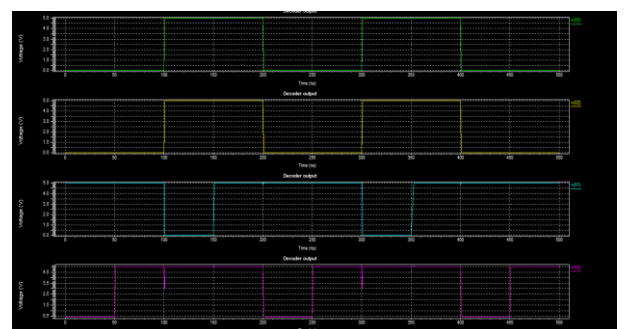
Fig.14.(b): Output waveform of decoder.
