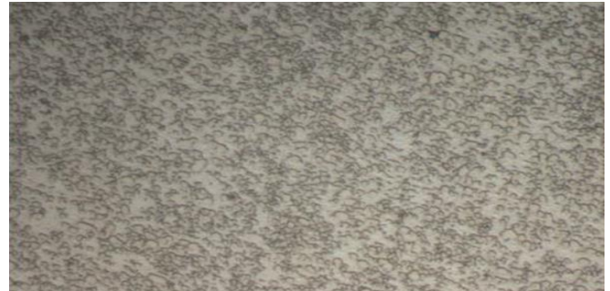
Figure 5. Microstructure of turned races at 1000x magnification
