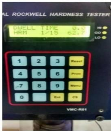
Figure 14(b): Hardness Test Reading on M scale
