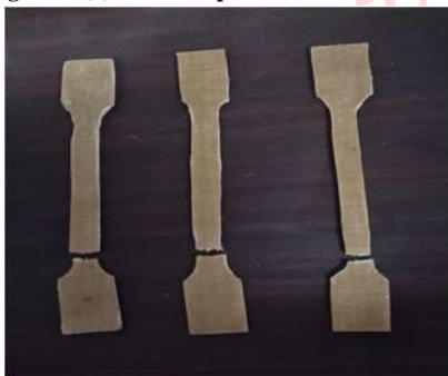
Figure 10(b): Tensile Specimen after Fracture
