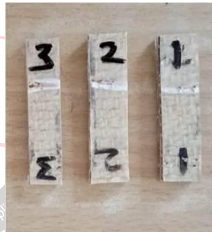
Figure 13(a): Impact Specimen Before Fracture
