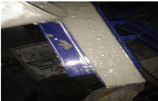
Fig.4 V funnel test
