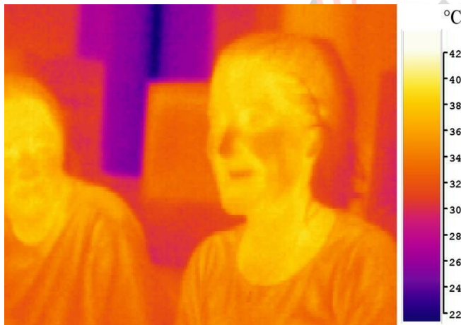
Fig.2: A pseudocolor image of two people taken in long-wavelength infrared (body-temperature thermal) light.
