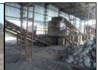
Fig-3 60 mm size of slag crushes upto 20mm size in 3 rd hopper
