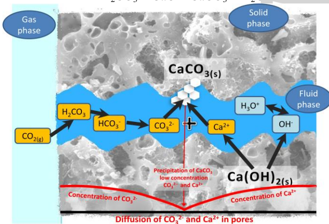
Fig-1: Carbonation mechanism in concrete.
