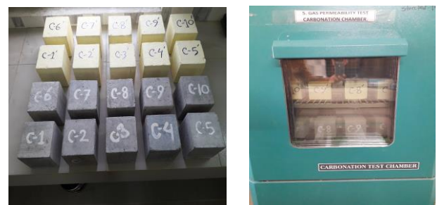
Fig-3: Concrete samples at Carbonation chamber.
