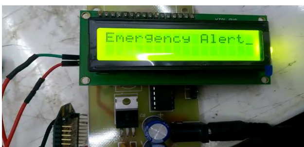
Fig. 6 Receiving Zigbee signal from transmitter
