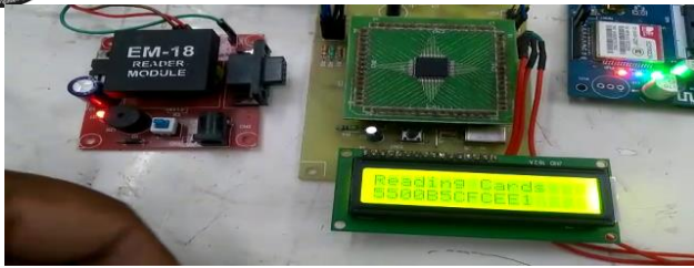
Fig.2 Reading RFID tags
