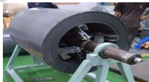
Fig. 1. Steel Insert on Jaw of Decoiler
