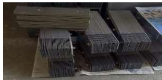
Fig. 2. Steel Out from Decoiler
