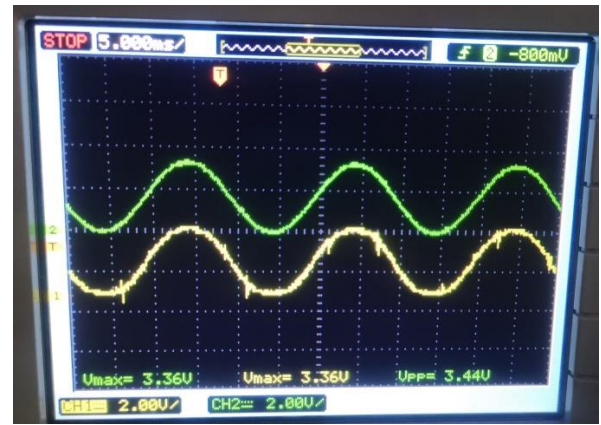
Fig.10.Reference voltage and output voltage waveforms
