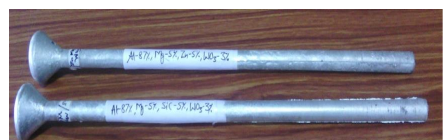
Figure 2 Casted cylindrical pins of MMC
