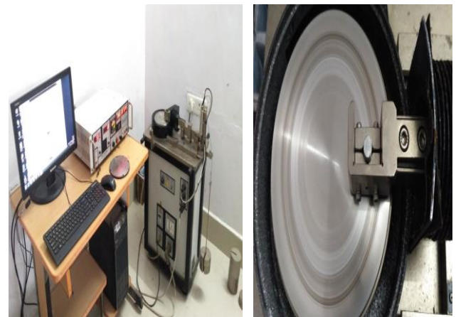
Figure 5 Pin-on-Disc dry sliding wear test of developed MMC
