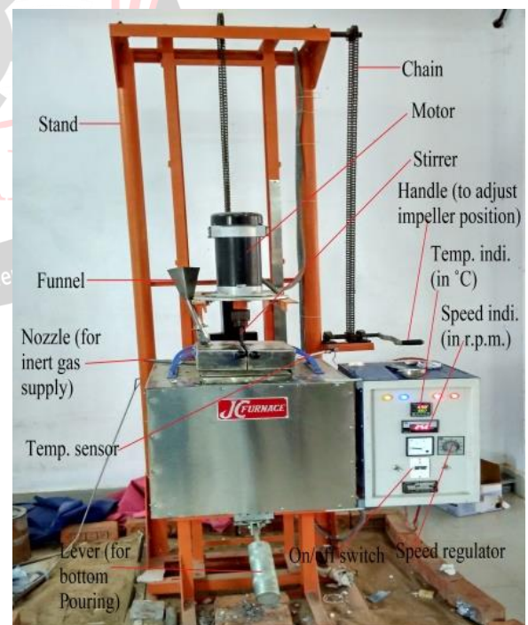
Figure 1 Setup of stir casting furnace
