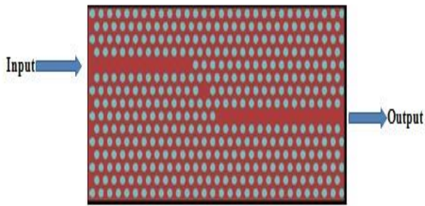
Fig.1.Schematic diagram 2D Photonic crystal Based pressure sensor
