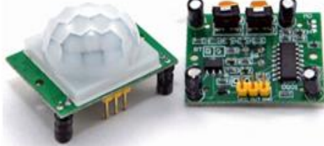
Fig 5. PIR motion sensor
