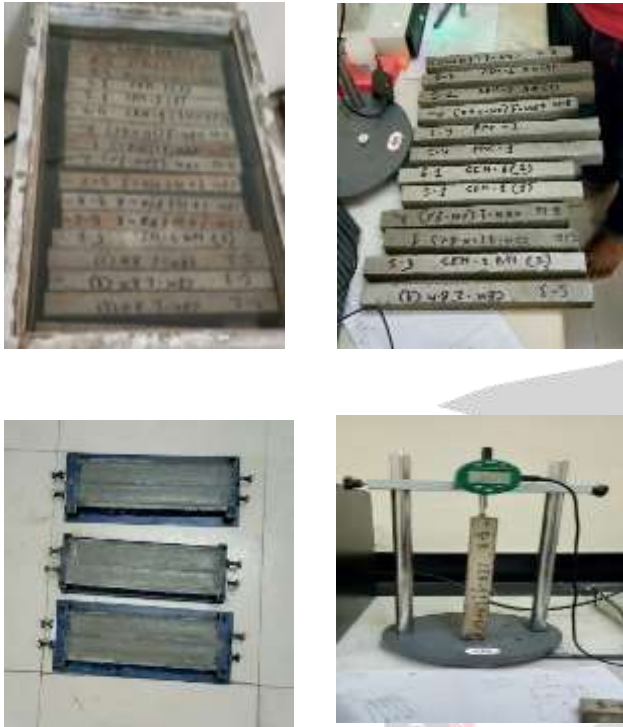
Fig. 1. Samples for ASR expansion test as per ASTM C1260.
