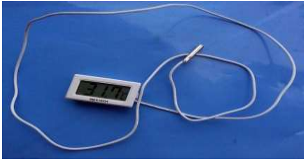
Figure 06: Figure of temperature indicator
