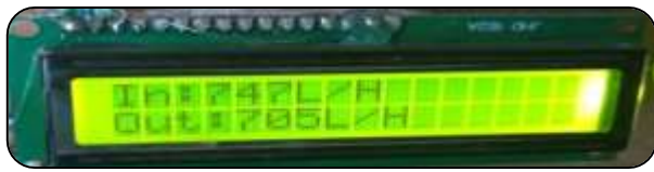
Fig. 12 Inflow and outflow data displayed in LCD
