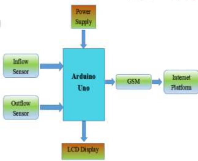
Fig. 3 Block diagram of water leakage monitoring system
