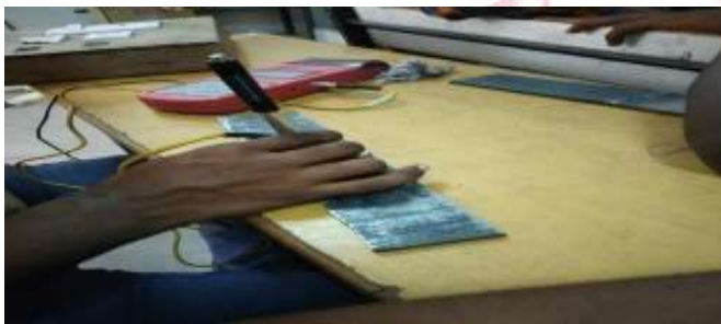
Hardness test After welding process
