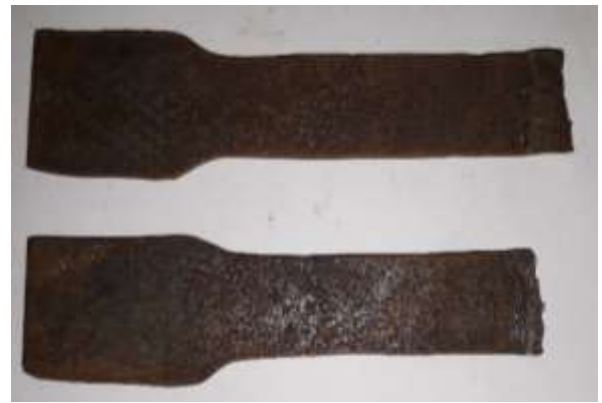
Fig: 5.2 Specimen of tensile test using high current
