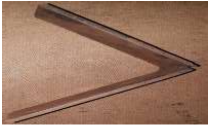
Fig: 5.3 Specimen after Bend test using low current
