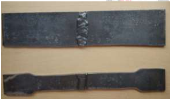
Fig: 4.2 Schematic of tensile specimen transverse section of weld joints
