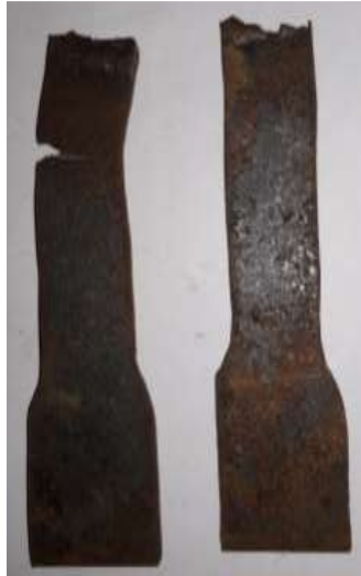
Fig. 5.1 Specimen after Tensile Test using low current
