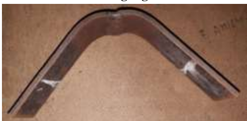
Fig: 5.4 Bending test of ms plate using high current
