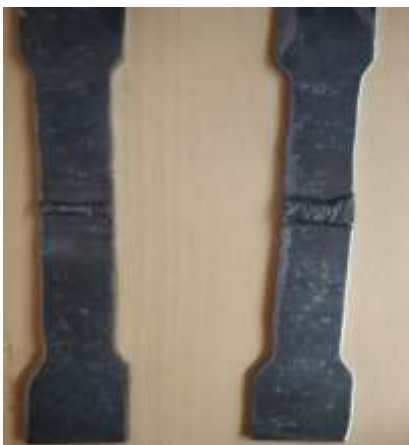
Fig: 4.3 Schematic of tensile weld metal specimen
