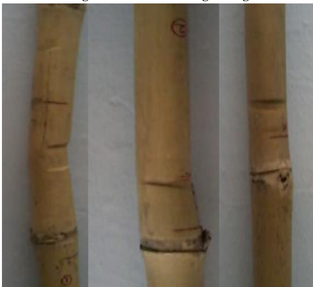
Fig. 2.5. C. Failure mode of sample observed after testing
