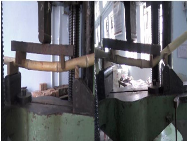
Fig.2.5.B. Failure during testing
