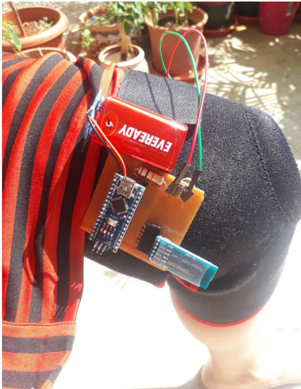
Fig. 5. Knee Flexion/Extension measurement system tied on the knee
