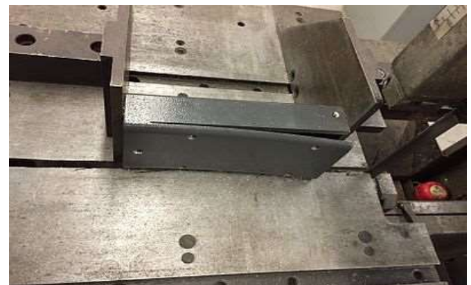
Fig1.4.1: Residual stress in a roll formed HSS tubing visible during band-saw slitting
