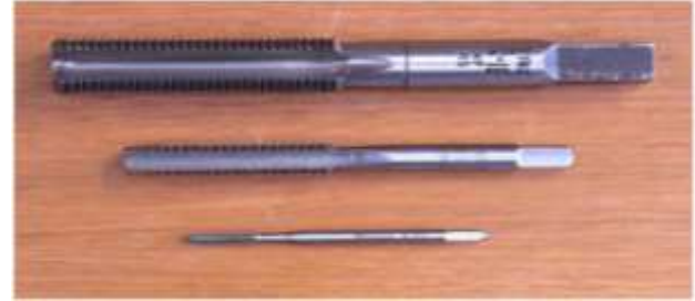
Figure 12: Taps used for this project
