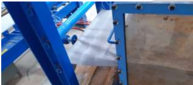
Fig 4- hydraulic jack for pulling geotextile
