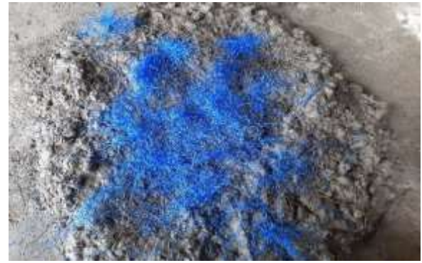
Figure 4. synthetic fibre & steel fiber concrete mix
