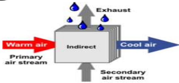
Figure 1: In-direct evaporative cooling system
