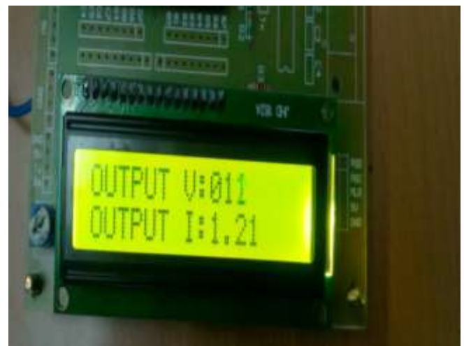
Fig.6.2 The experimental hardware effects of proposed controller one LED to 2nd LED flip on cutting-edge is 1.20A continuously maintained.
