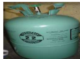
Fig. 8: Cylinder of R-22 refrigerant
