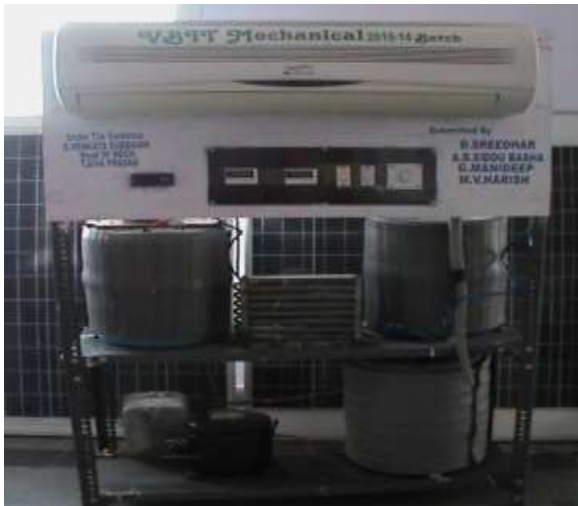
Fig. 12: Fabrication Of Hot & Cold Water Cum Air Conditioning System
