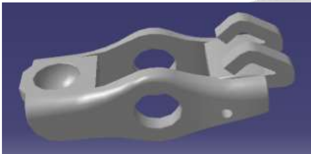
Fig - 3: Model of Rocker Arm after Modification
