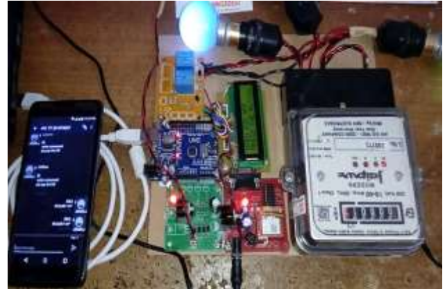
Fig.4: Smart Energy Monitoring system using Android Application
