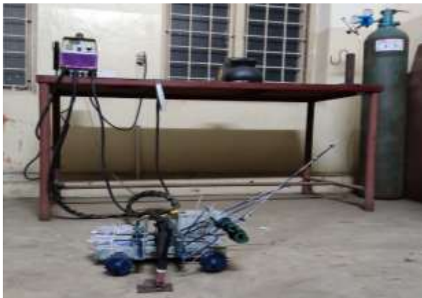
Fig. 1 A photograph showing the TIG welding carriage with torch holder and wire feeder.
