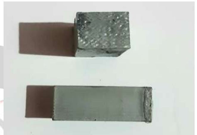
Fig 2. Acetone Dipped ABS Samples
