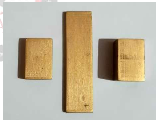
Fig 3. Copper Spray Painted ABS Samples
