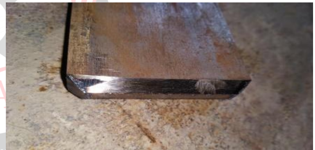
Fig.1- Edge Preparation by Grinder
