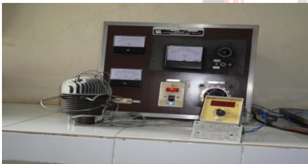
Fig. 3 Photographic view of the set-up to measure the surface temperature of liner and cylinder head
