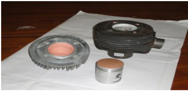
Fig. 1 Photographic view of copper coated piston, liner and copper coated cylinder head
