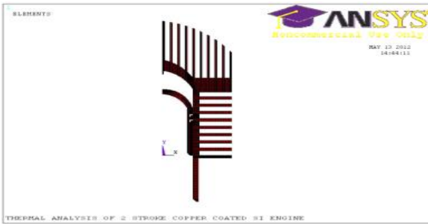
Fig. 7 Mesh employed in the thermal analysis for the assembly of copper coated piston, liner and copper coated cylinder head
