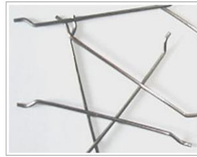
Flatted shape Steel Fibre with Hook (Figure1.3) [15]
